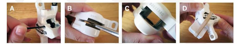
Now you'll need to place something between the pistons to keep them in that position throughout the bleed process. Anything of the correct size will do as long as it's not a compressible object (e.g. a piece of wood or plastic) and secure in place with the elastic band. (D)
